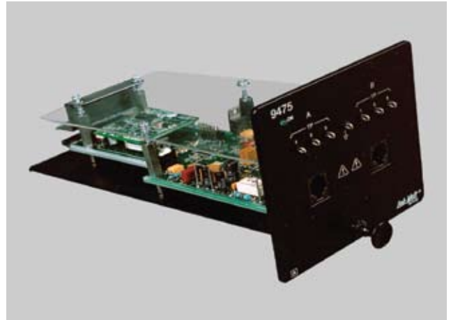
The Dual Analog Line Interface, Model 9475, is a simple interface card (module) to be installed in the reconfigurable Training Module, Model 9431. Two conventional telephone sets can be connected to this module.
