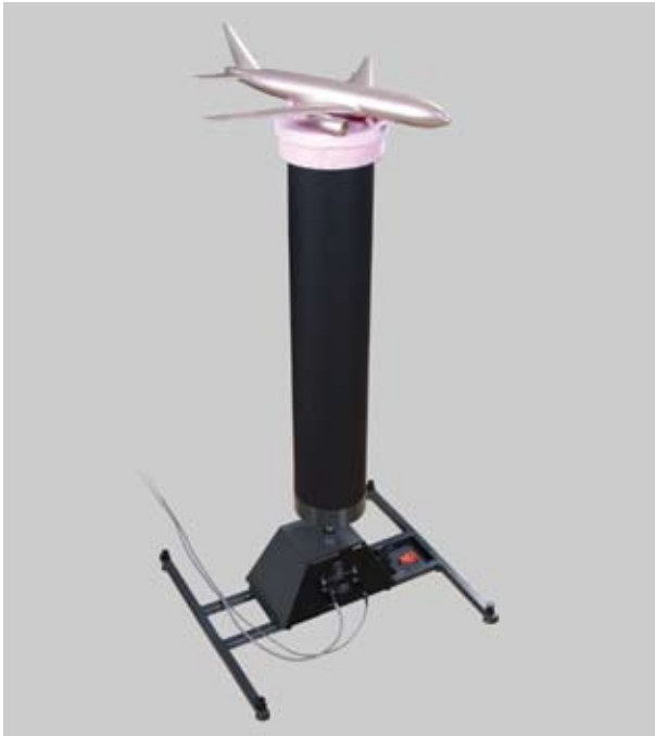
The RCS pattern of an actual aircraft can be obtained by placing a reflective scale model on top of the low-RCS rotating support of the RCS and ISAR Measurement Training System.
